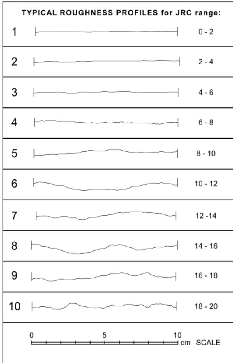
ISRM, 1981, Fig 17 Typical roughness profiles and suggested nomenclature. The length of each profile is in the range 1 to 10 metres. The vertical and horizontal scales are equal.
